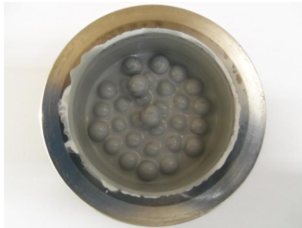
Fig. 3. Rock material after 1 h of wet ball milling using 50 wt% ethanol as PCA.
