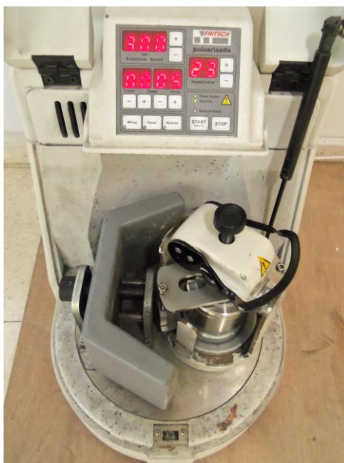
Fig. 1. The planetary ball mill that will be used during the CO2NOR Project (Fritsch Pulverisette 6 planetary mono mill).
